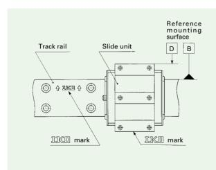
Fig. 5 Reference mounting surfaces
