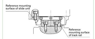
The reference mounting surface of track rail is made opposite to the standard side. The accuracy of dimension N including parallelism in operation is the same as that of standard specification.
