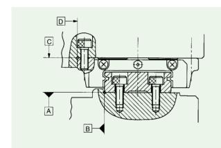
Fig. 4 Reference mounting surfaces and general mounting structure
