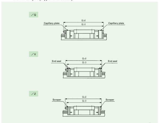
unit: mm With capillary plates (/Q) With double end seals(1) (/V)With scrapers(1) Model number L<sub>1</sub> L4 *L*<sub>1</sub> L4 L<sub>1</sub> L4 LWFF 33 64 67 61 64 62 64 LWFS 33 LWFF 37 73 75 70 74 71 75 LWFS 37 LWFF 42 86 99 82 96 84 97 LWFS 42 LWFF 69 121 133 117 130 119 131
