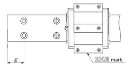
The mounting hole positions of track rail can be specified by specifying dimension E at the left end, which is the distance from the mounting hole nearest to the left end of the track rail to the left end face of the track rail in sight of TIKO mark on the slide unit.
