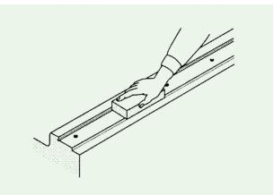
Fig. 7 Cleaning of mounting surfaces
