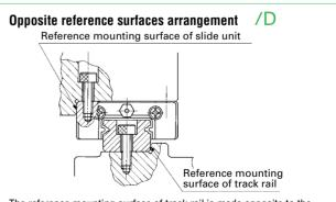
The reference mounting surface of track rail is made opposite to the standard side. The accuracy of dimension N including parallelism in operation is the same with that of standard specification.
