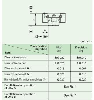
Note(1): It means the size variation between slide units mounted on the same track rail.
