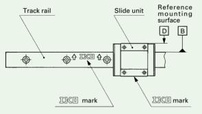
Fig. 5 Reference mounting surfaces
