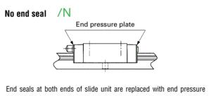
End seals at both ends of slide unit are replaced with end pressure plates that are not in contact with the track rail to reduce frictional resistance. The under seals are not assembled.
