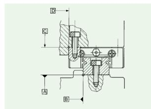
Fig. 4 Reference mounting surfaces and general mounting structure
