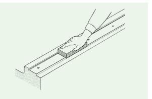
Fig. 6 Cleaning of mounting surfaces
